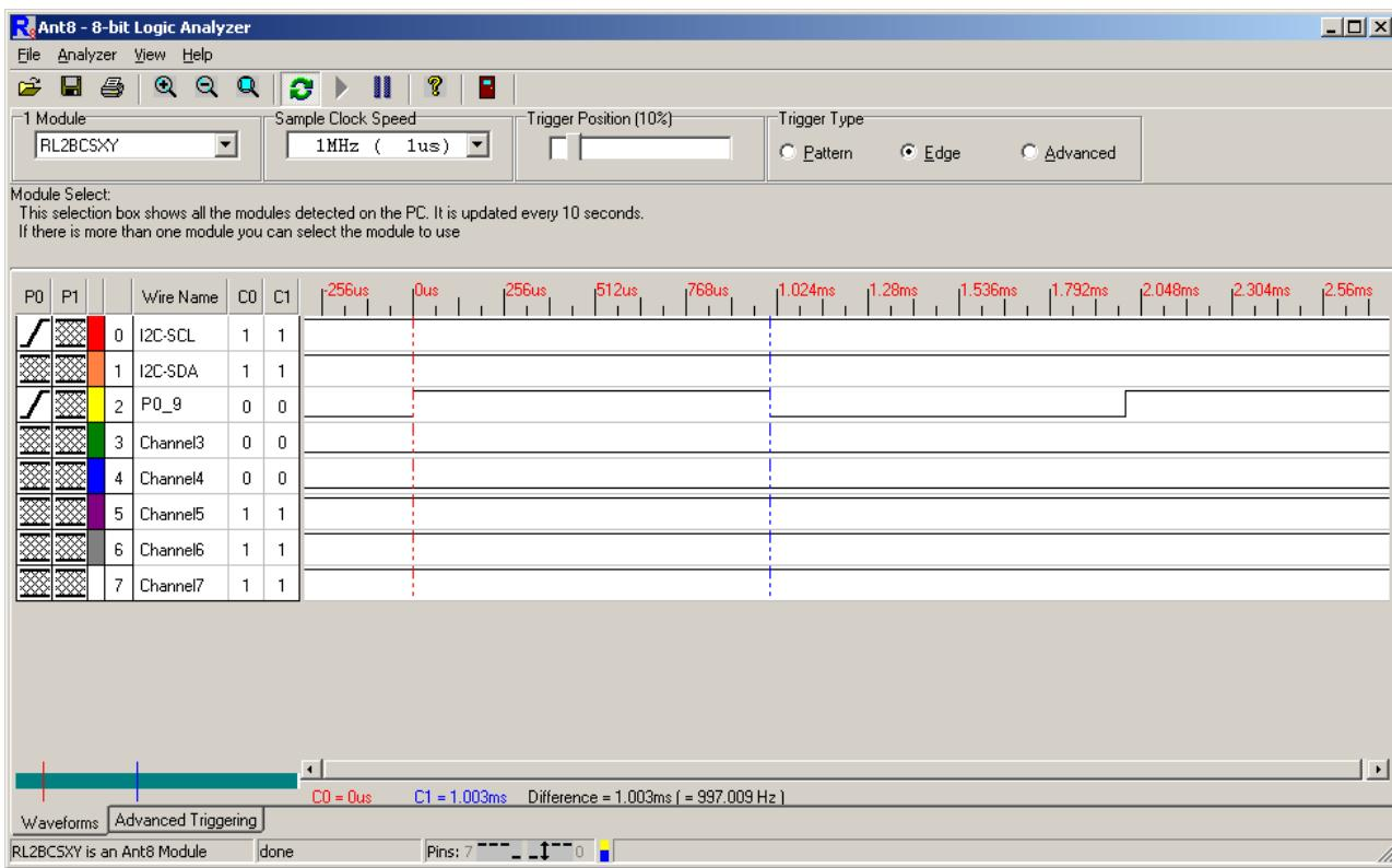
The following waveform capture shows the 10 mS delay:
