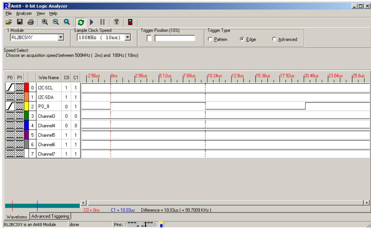
The following waveform capture shows the 100 uS delay:
