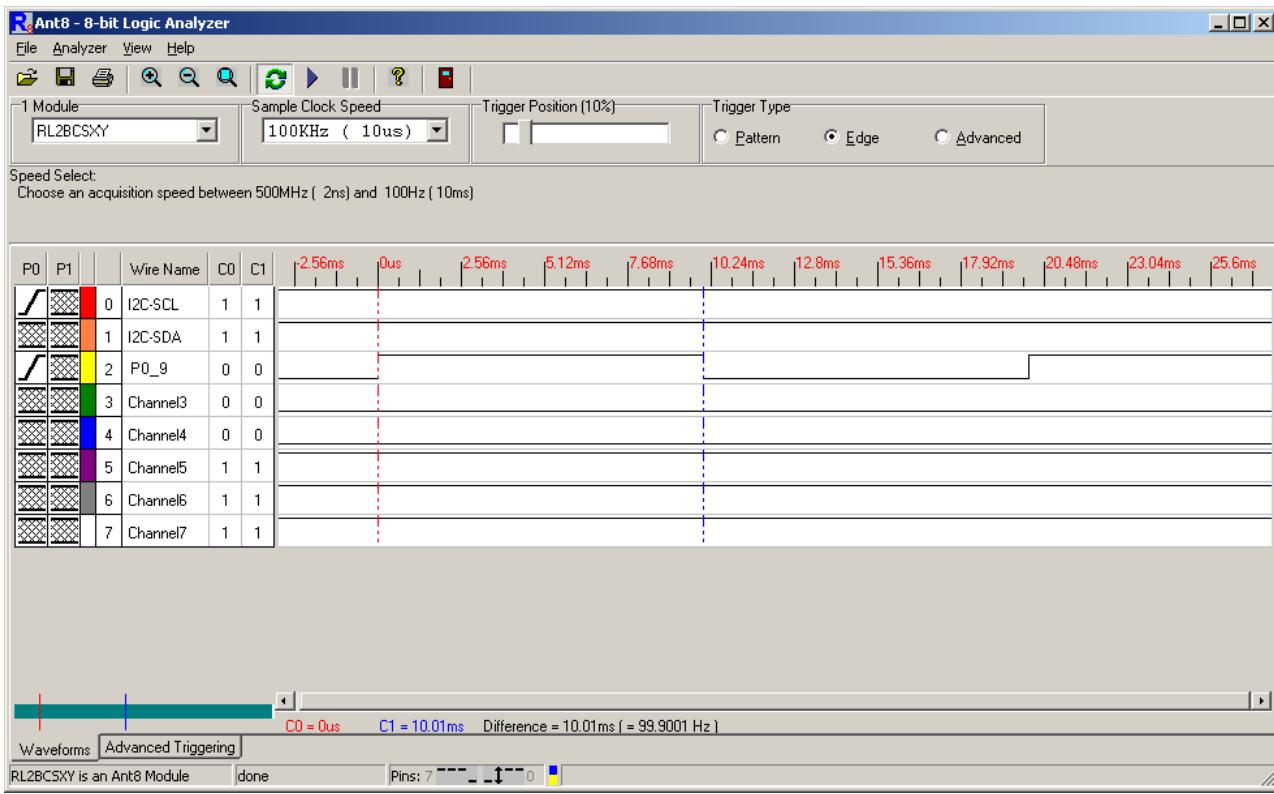
The following waveform capture shows the 100 mS delay:
