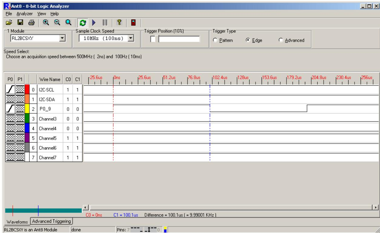
The following waveform capture shows the 1 mS delay:
