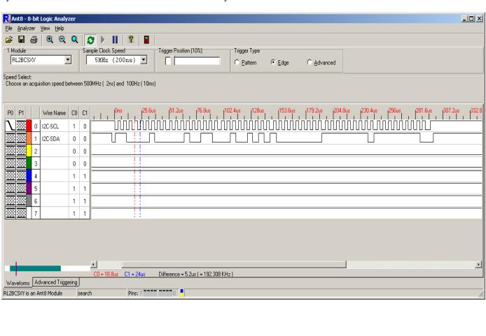
The following waveform capture shows 2 bytes for a read from the PCA9551 by the MicroBolt over the I<sup>2</sup>C bus. The first byte is the PCA9551 slave address of 0x61 and the next byte is the input register status of the PCA9551.
